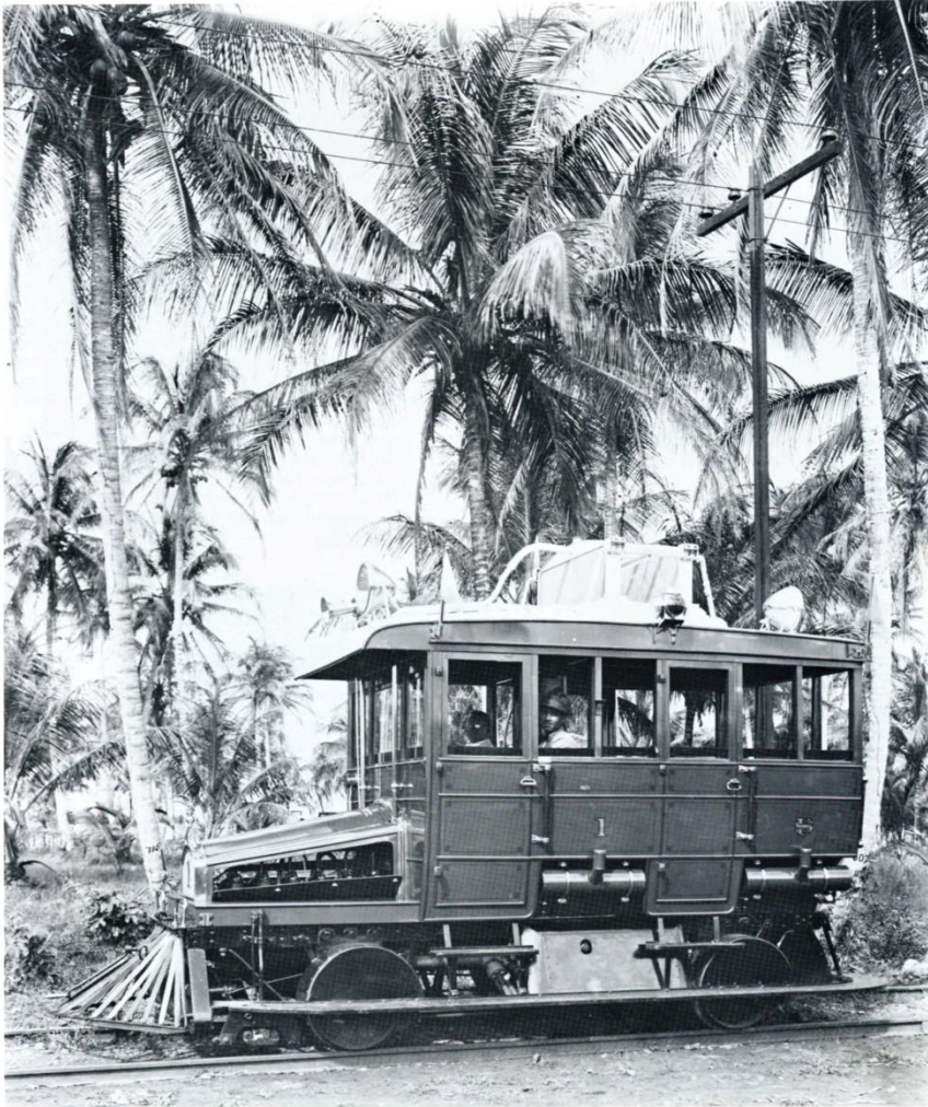
The rail motors had all of the equipment to qualify as a train under the standard book of rules. A six cylinder gasoline engine drove the rear axle. This car was built by the Stover Motor Car Company of Freeport, Illinois during 1908. PCC 1538
